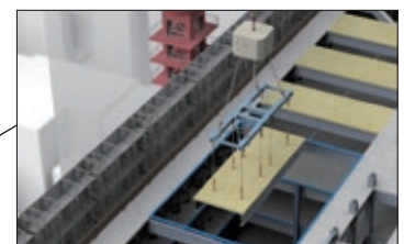
(3) Each block is lowered through a large opening inside the building and broken down into small pieces on the ground floor.
