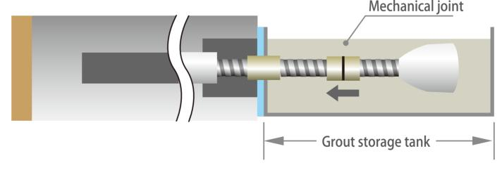
Construction drawing with mechanical joint
