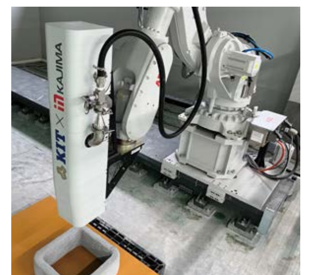
An example of mortar layering status
