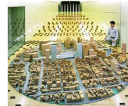
Evaluation of wind environment around tall building (using wind-tunnel laboratory)
