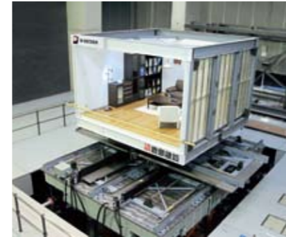
Reproduction test of the seismic response of a high-rise building
