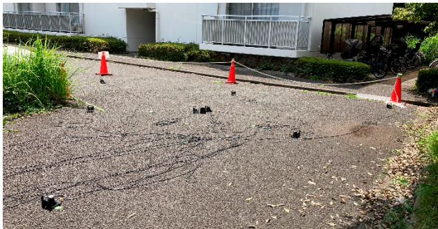
Photo 2 浅部地盤の微動探査時のセンサー配置例 (Example of Sensor Installment for Investigating Shallow Underground Structure)
