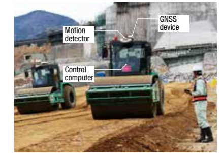
General-purpose vibrating roller equipped with a control computer and automatic steering
