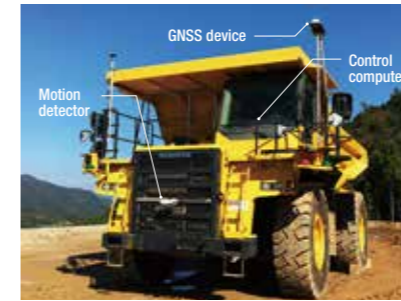
General-purpose dump truck equipped with a control computer and GNSS device
