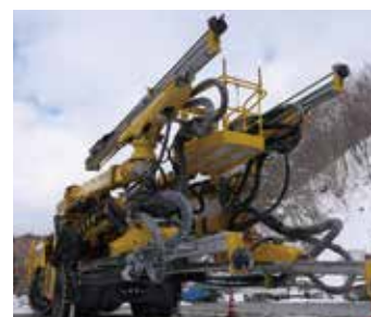
Kajima utilized the Four-Boom Full Auto Computer Jumbo for the main boring of the Shinkuzakai Tunnel in Iwate Prefecture, a first in Japan. Going forward, the aim is to automate the entire series of operations related to tunnel construction.
