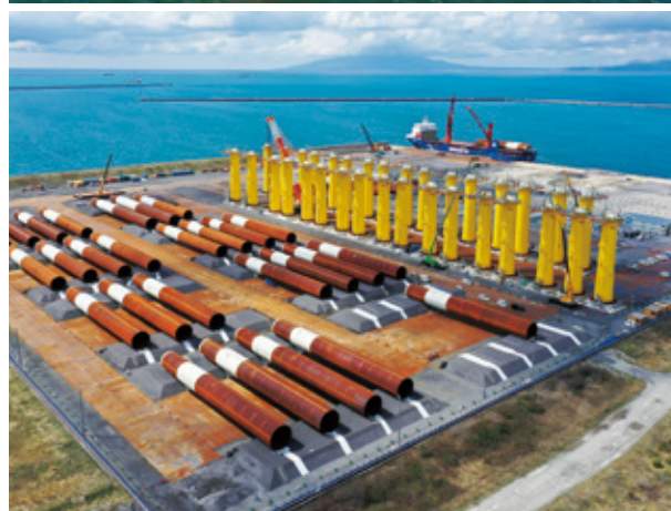
Akita Port & Noshiro Port Offshore Wind Farm Projects (Above) SEP vessel in operation (Below) Panoramic view of the pre-assembly yard for wind turbine foundations
