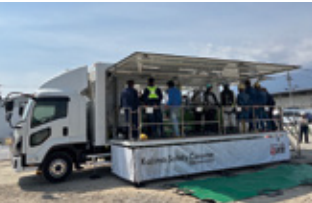
Left: The training vehicle is a mid-sized (11t) truck equipped for nine types of hazard simulation training Right: An employee in a VR hazard simulation training program
