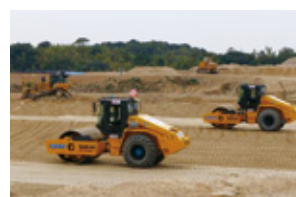
Collaboration work by two rollers modified for automation (Okazaki Achiwa Industrial Park land development project) Details can be checked using the above 2D code.
