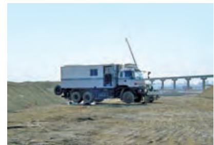
Soil strata survey using the Geo-Explorer truck
