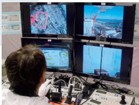
To eliminate the need for on-site workers, cranes in highly radioactive locations are operated from this control room.
