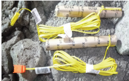
Photo 2 高精度電子雷管 eDev II と含水爆薬 (eDev II and Cartridge Type Explosives)
