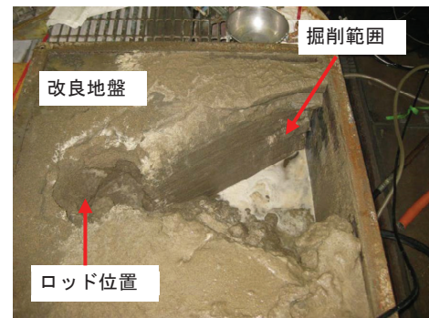
Photo 7 固化後の掘削 (Excavation after Solidification)
