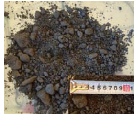
Photo 7 造粒固化物 (Soil Like Material) produced from Cemented Fly Ash
