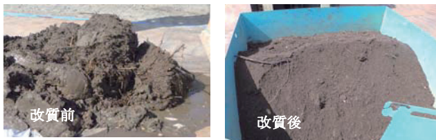
Photo 4 泥 DRY による除染土壌の篩分け選別状況 (Sorting Plants from the Removed Soil)
