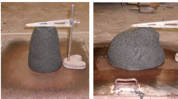
Photo 3 自立状態 (左) と塑性流動状態 (右) の土砂 (Soil of the Self-Supported State (left) and the Plastic Fluidized State (right))
