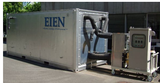
Photo 1 炭酸化養生設備 (Carbonation Curing Chamber)
