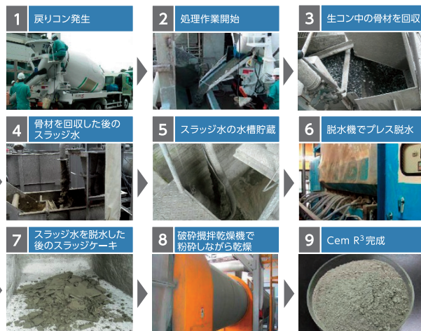
乾燥スラッジ微粉末(CemR 3 , DSP)の製造工程 Manufacturing Process of Dehydrated Sludge Powder
