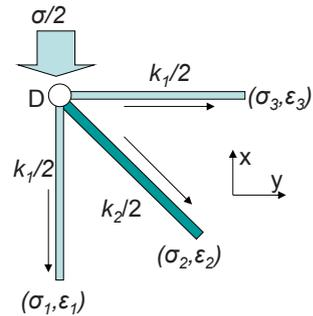
Fig.7 D点の応力 (Stress at Point D)
