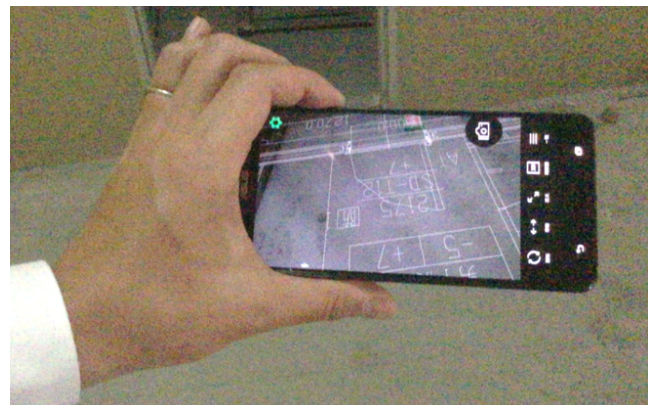
Fig.6 Overlay of 2D Image on Floor for Grid Inking Task
