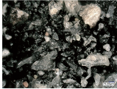
Photo 1 しらす土粒子 (顕微鏡 200 倍) (Scanning Electron Microscope Image of Shirasu Soil Particle, 200x)
