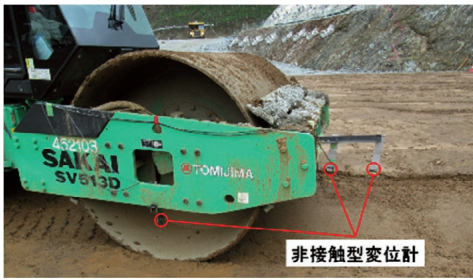
Photo 3 大型ローラと非接触型変位計 (Large Roller and Non-Contact Displacement Sensor)
