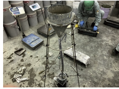
Photo 1 供試体の作製概要 (Outline of Preparation of Specimen)
