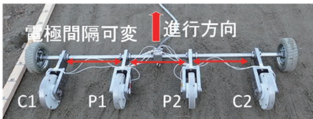
Fig.6 車輪型電極 (System Integration for Soil Resistivity Measurement using Wheel Type Electrodes)
