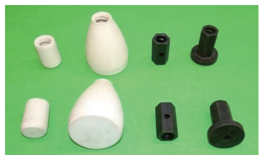
Tip anchor End anchor Tip anchor End anchor (a) Ceramic (b) Steel
