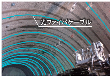
光ファイバによるトンネル支保応力計測 Measurement of Tunnel Rock Support Stress by Distributed Fiber Optic Strain Sensing
