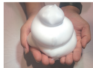
Photo 1 気泡 (Foaming Agent for EPB TBM)
