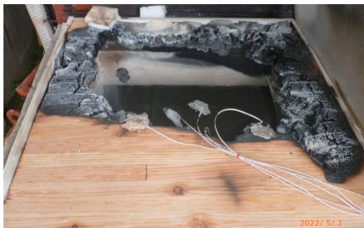
Photo 7 加熱試験後のカラマツ板, No.5 (Larch Board after Heating Test, No.5)
