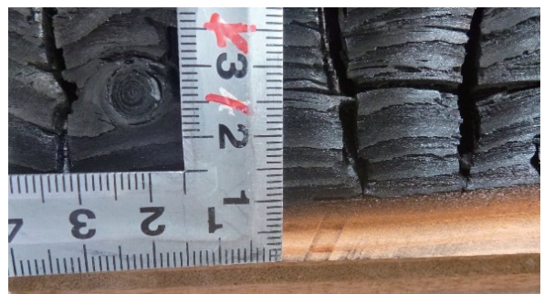
Photo 9 加熱試験後の残存厚さ, No.6 (Residual Thickness after Heating Test, No.6)
