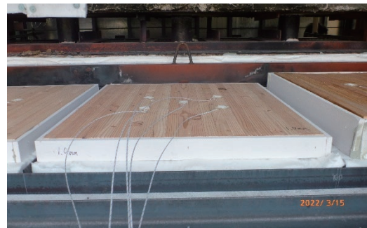
Photo 4 加熱試験の裏面状況 (Test Situation of Heating Test)
