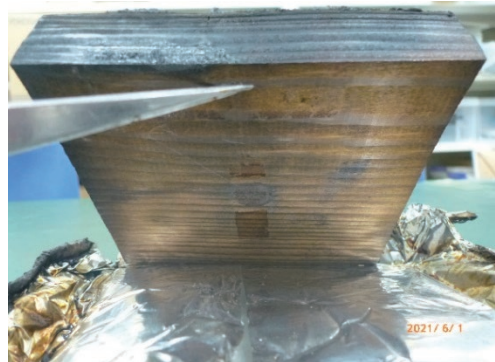
Photo 3 試験後の裏面状況, No.7 (Back Side Condition after Cone Calorimeter Test, No.7)
