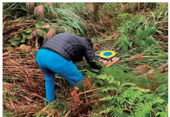
Photo 5 GNSS内蔵対空標識設置状況 (Installation of Anti-aircraft Sign with Built-in GNSS)
