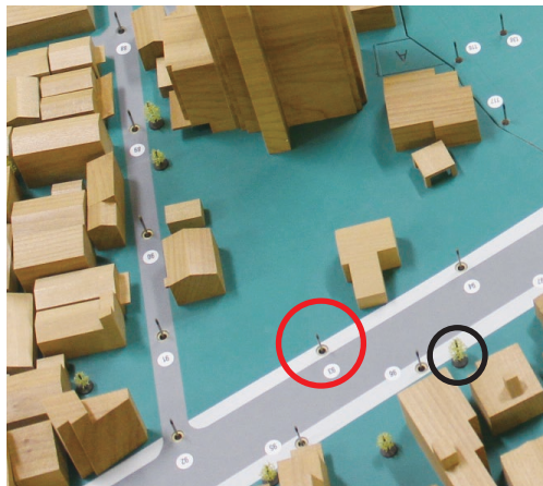
街区中の多点同時風速計(赤丸:風速センサー,黒丸:樹木模型) Multi-anemometers in Urban Area (Red circle: anemometer, Black circle: tree model)
