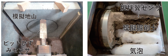
ビットひずみセンサ(左)と攪拌翼センサ(右) Cutter Bit Strain Sensor (left) and Stirring Blade Sensor (right)
