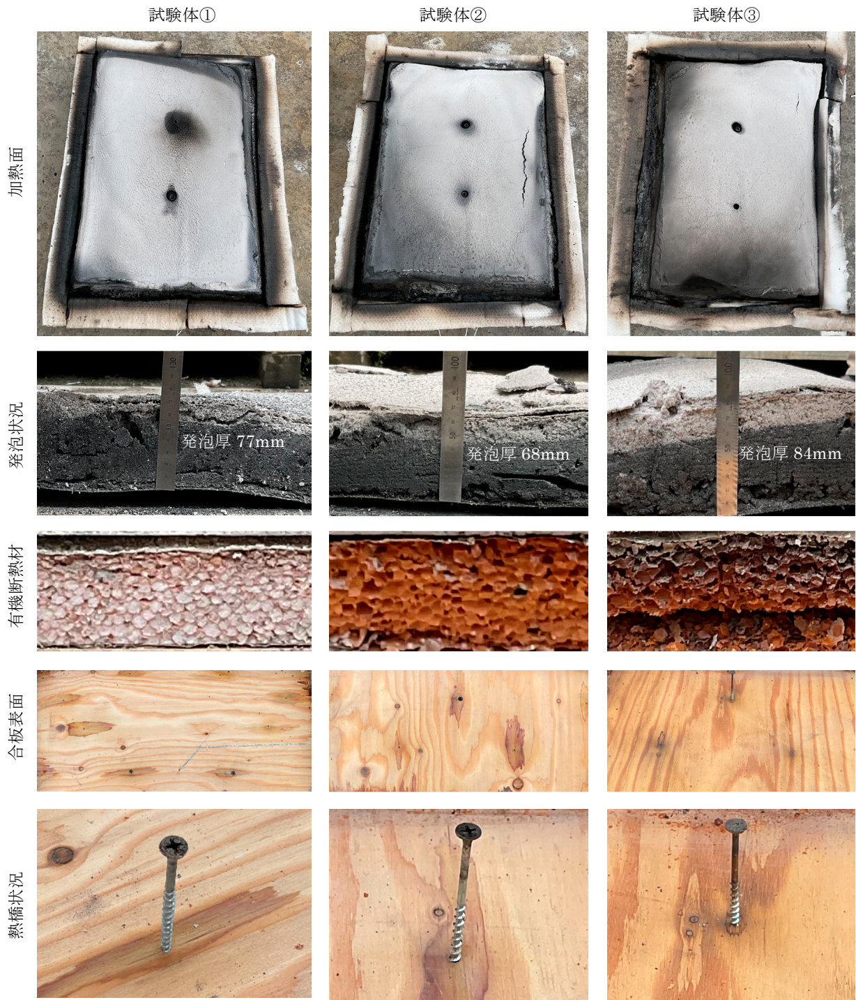
Photo 7 試験後の試験体の状況 (Specimen after Heating Test)
